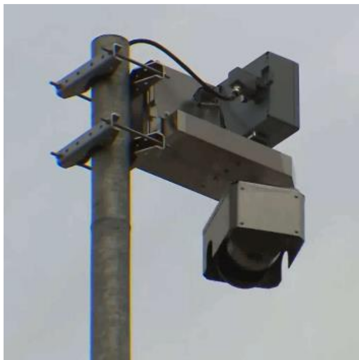
Figure 20: Detection of parking trucks by laser scanner
