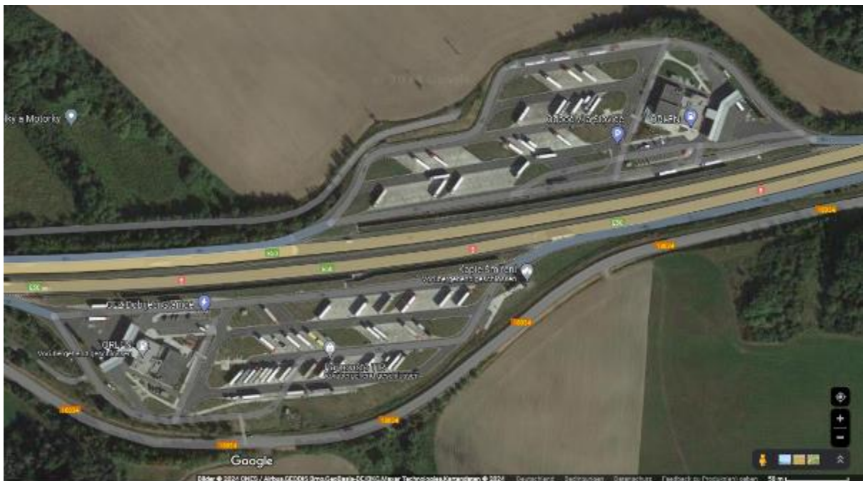
Figure 11: Example for a big parking site at the D5 with a classical arrangement of parking places in three rows.
